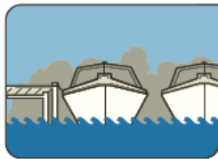
"Station wagon" effect or backdrafting at low speeds
